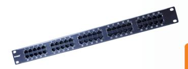
D-Link Voice patch panels are high density patch panel with 50 RJ45 ports on 1U applied and suitable for 22-26AWG stranded and solid wire, compatible with both 110 & Krone punch down tools. D-Link patch panels have improved Cable Management with optional Cable Management bar terminating 4 pairs UTP cable. They are complied with the FCC Part 68 sub part F standard.
